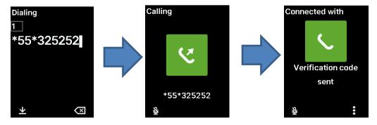
2 The handset will return "Verification code sent" in the handset's display, and will hang-up after 10 seconds.
