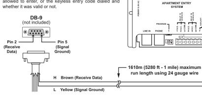
If the RS-232 input of a PC, printer, etc. is capable of receiving TTL level RS-232 signals, then the LOG BUS can be wired directly into the RS-232 "Receive Data" and "Signal Ground" pins to receive ASCII data. Windows "Hyper-Terminal" can be used to receive the data on a PC (use the settings in the chart) or visit www.vikingelectronics.com to download free ENTRY LOGGER software (see Operation section E, "Entry Logger Software").
