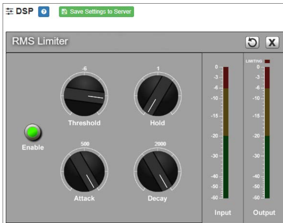
Figure 19. RMS Limiter Settings
