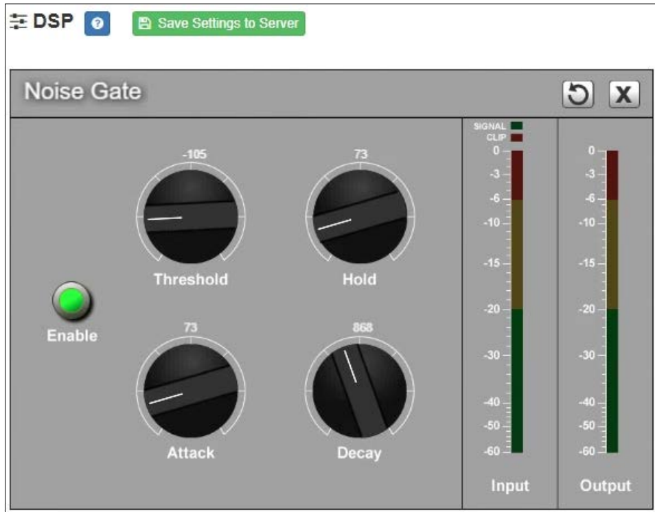
Figure 15. Noise Gate Settings
