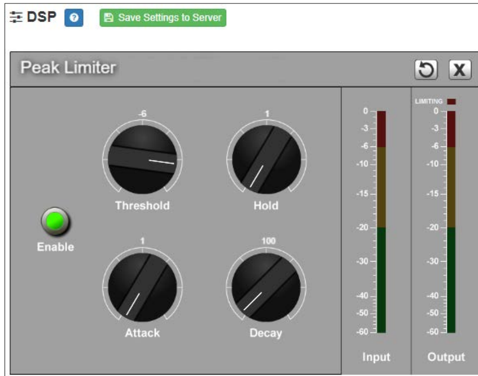
Figure 17. Peak Limiter Settings
