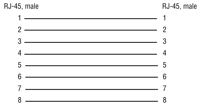
Figure 9. Typical Ethernet straight-through cable diagram for 1000Base-T
