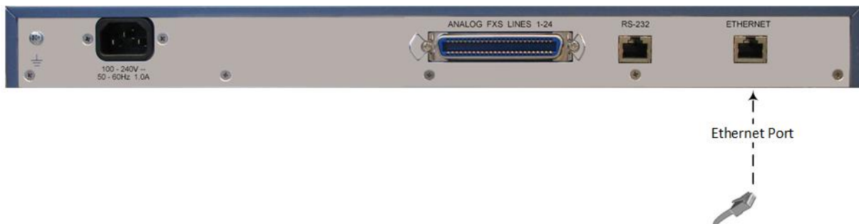
Figure 5-4: Connecting Device to Ethernet Network
