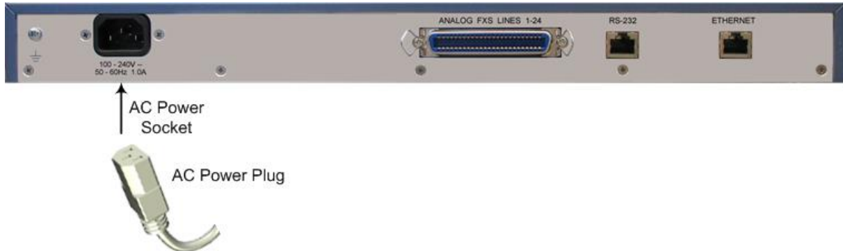
Figure 5-23: Connecting Device to AC Power Supply
