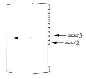
Attach the cover to the base with the two included screws as shown.
