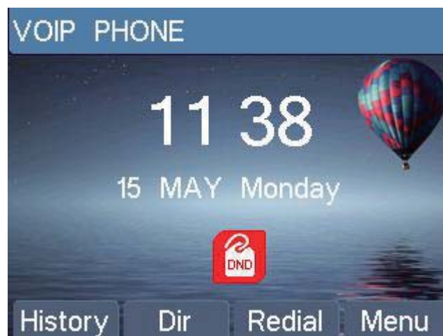
Figure 56 - DND Enabled on All Lines
