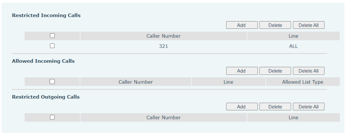
Picture 97 - Web Blocked List
