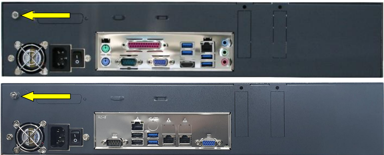
Figure 1: Grounding Screw on CXR2000/CXR3000 Rear Panels
