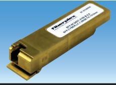
FiberPlex SFX-DD Data Diode SFP Modules for cyber security, with gigabit or 10-gigabit optics, transmit data in one direction only without the possibility for a return path, making them ideal for applications such as file transfer, real-time data streaming, database replication, and remote monitoring.
