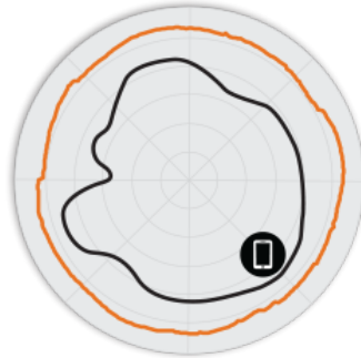
Figure 3. R750 5GHz AzimuthAntenna Patterns
