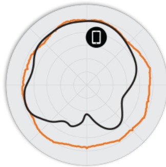
Figure 3. R320 5GHz Azimuth Antenna Patterns
