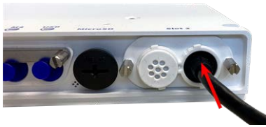
Fig. 35: Press the plug in firmly until the blue sealing ring clicks into place
