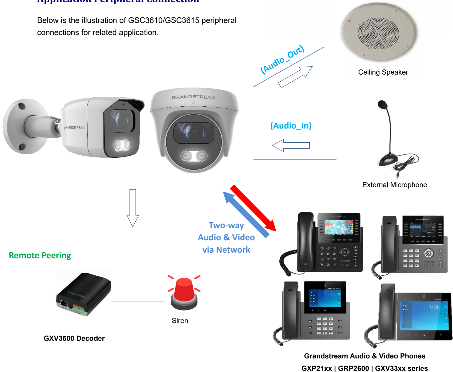
Figure 7: Application Peripheral Connection for GSC3610/GSC3615
