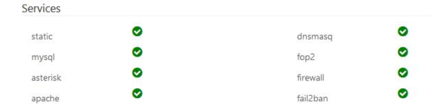
This section displays the current status of all the services associated with the TwinStar cluster. All services that are behaving correctly will be shown with a green  $\checkmark$  symbol. Any service that is not behaving in the correct manner will be shown with a red  $\checkmark$  symbol.
