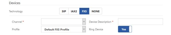
**Channel\***, the DAHDi channel, selected from the drop-down list, that should be associated with this device.
